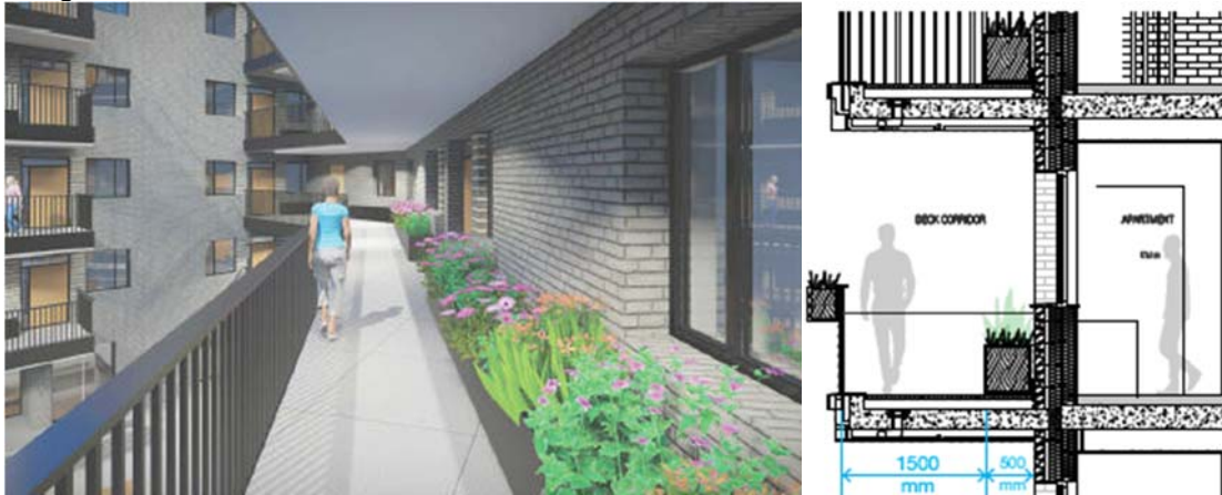
Image 26 & 27: deck access visual and section
